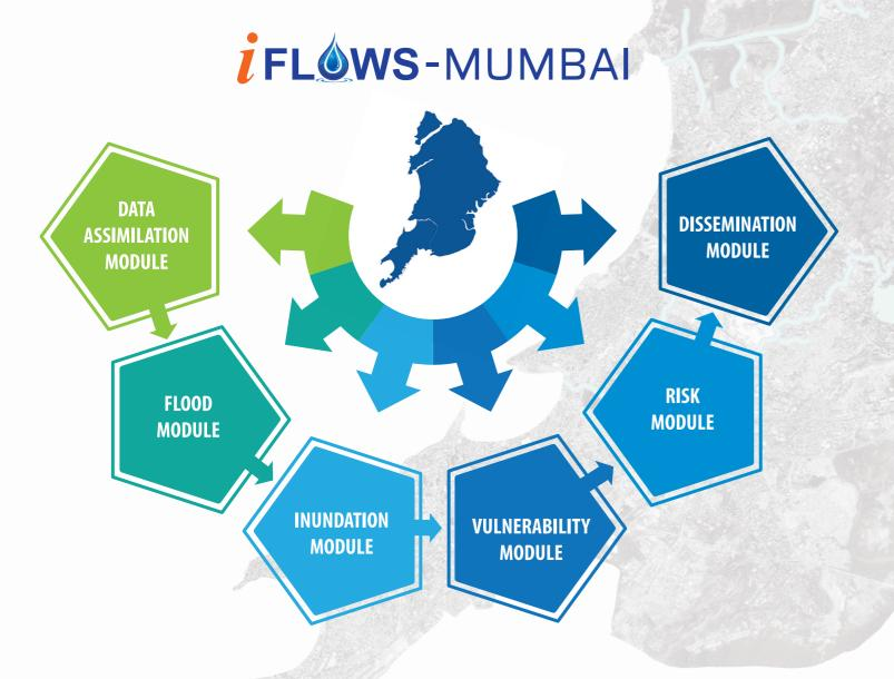
iFLOWS-Mumbai will address the flood inundation due to rainfall, river bank breach, storm surge, obstruction of flow due to road, railway, buildings etc., high tides and sea level rise. The system will be useful in planning flood mitigation measures such as retaining walls, improvement in storm water drainage system, locations for pumping station and operation of lock gates in the rivers and lakes etc.
